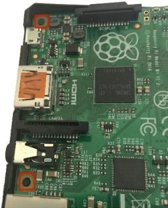
1. Line up the hdmi side of the Pi with the lower half of the case and ease it into place at a slight angle pressing down gently but firmly until the mounting posts (highlighted in red) click into place in the Pi's screw-mounting holes.
